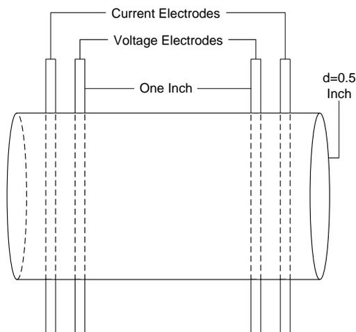
Picture of Setup / Figure of Test Apparatus
