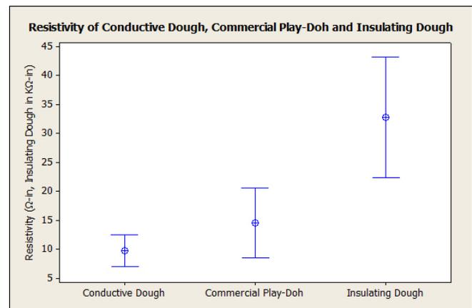
Comparison of Three Resistivities (Note that Insulating Dough is Measured in Kilo-Ohms)
